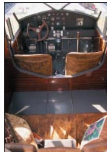
Two forward and two or three aft is the seating arrangement of the S-39.
